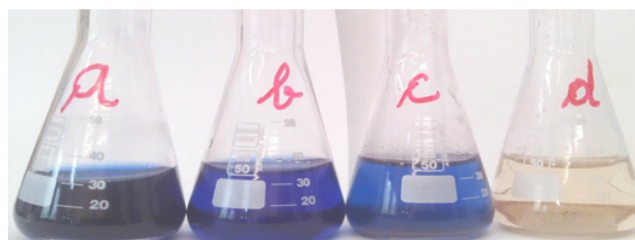
Fig. 5. Visual presentation of BB 41 solutions at 24 hours: untreated (a); discolored with \text{H}_2\text{O}_2 (b), HAp/Ag (c), and HAp/Ag/ \text{H}_2\text{O}_2 (d)
